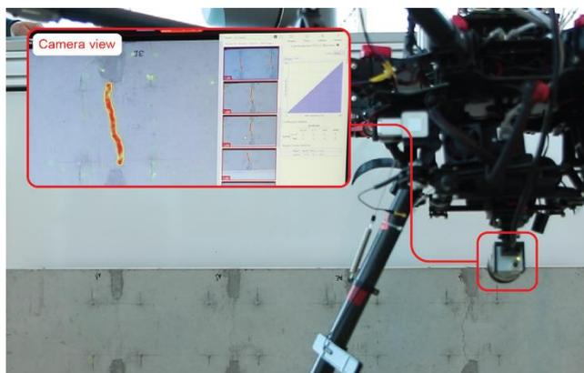
**Fig. 3:** AI-based crack detection system tested in controlled environment at Teknologisk Institut.
