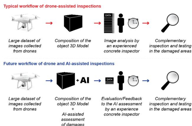
**Fig. 4:** The future of concrete damage assessment – Drone and AI-assisted inspection workflow.
